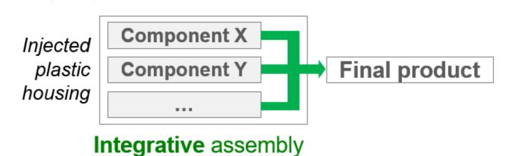
(The injection moulding process realizes the assembly)
