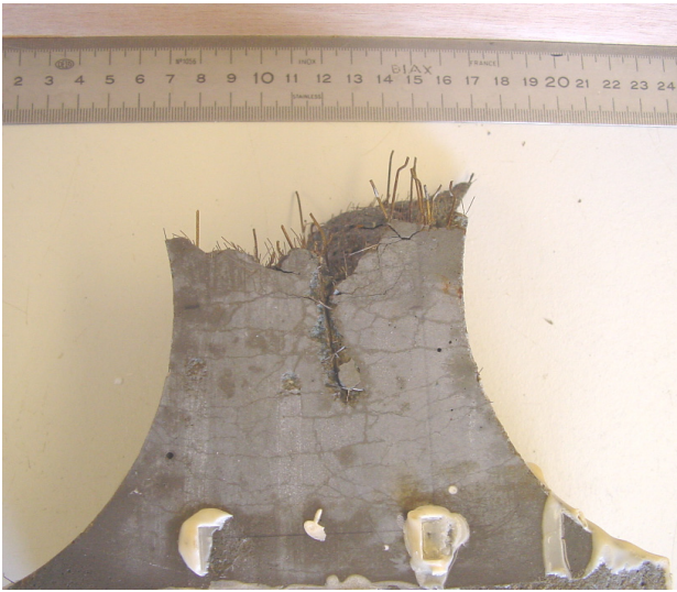
Fig. 4. Hardening behaviour of a mixture with 1Vol.-% long (60/07) and 0,5Vol.-% short (13/0,2) fibers [2].
